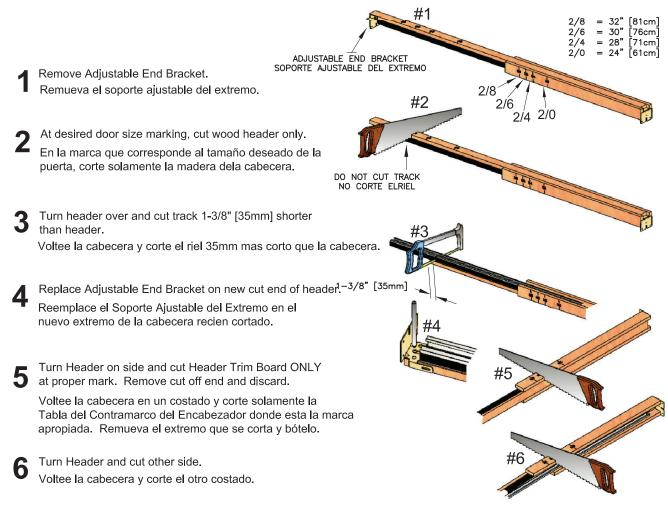
Cutting header for other than standard door width: Measure door width and multiply by 2. Add 1" (25mm). Mark header and cut (Step #2). Cut track (Step #3). Measure door width. Add 1" (25mm). Mark header Trim board and cut (Step #5 & #6).
