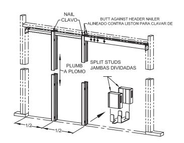
Apply desired wall material. Wall material is brought clear to edge of opening. WARNING: Use nails no longer than necessary. Nails must not protrude into pocket or door will be damaged. To provide a firm nailing surface, slip a 2-1/8" (54mm) wide board between Split Studs temporarily.
